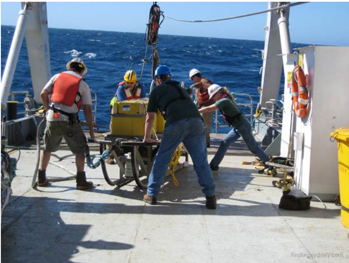
Above: steadying the sonar towfish to be lifted off the deck
