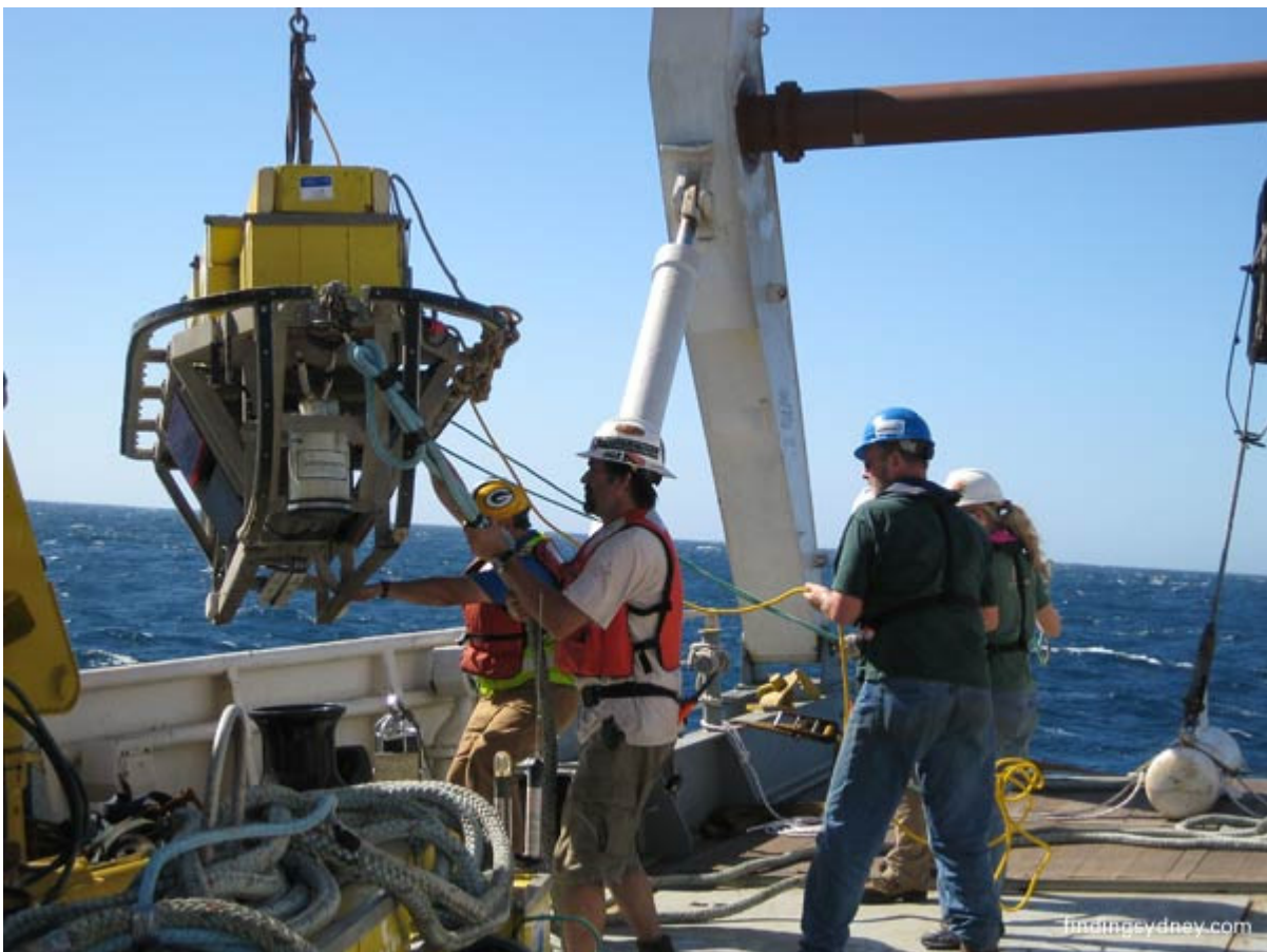
Above: steadying the sonar towfish to be lifted off the deck
