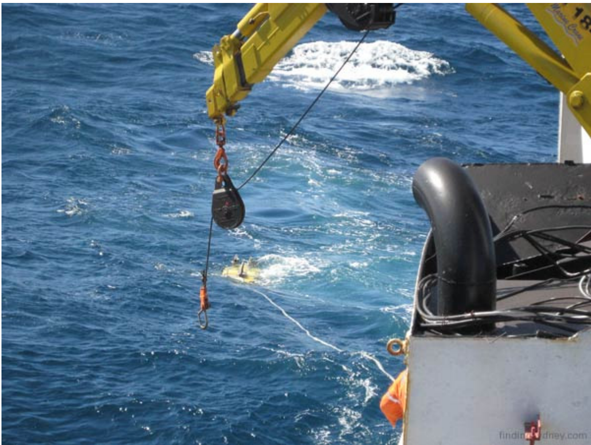
Above: streaming the towfish behind the ship, and finally
